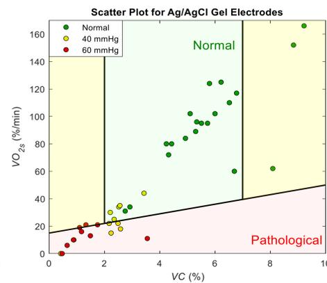
Scatter plots for textile band and Ag/AgCl gel electrodes: the sensitivity was 40% for band and 72% for gel electrodes, with specificity at 100% for both. Samples that fell into yellow areas were ignored.
