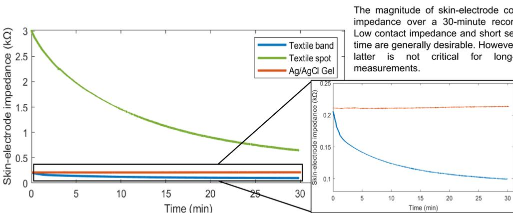
The magnitude of skin-electrode contact impedance over a 30-minute recording. Low contact impedance and short settling time are generally desirable. However, the latter is not critical for long-term measurements.
