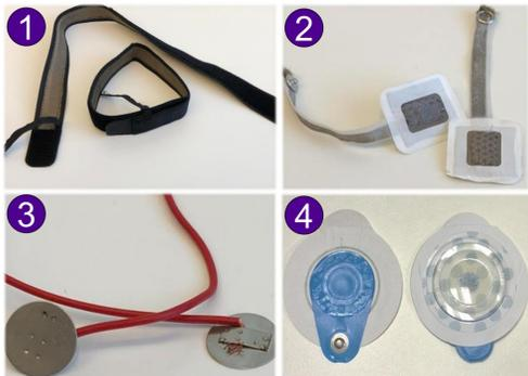
Evaluated electrodes: 1) Textile band 2) Textile spot 3) Metal plate 4) Disposable Ag/AgCl gel electrodes
