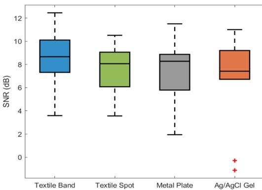
SNRs for each electrode type. No statistically significant differences were found ( $p > 0.05$ ). Values deviating from the median more than 1.5 times the interquartile range, have been marked with red sign.
