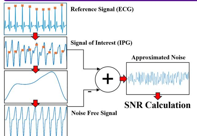
SNR calculation from impedance plethysmography (IPG) signal using template matching.
